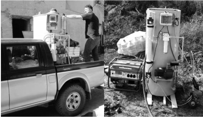
Photo: Preparation for transportation of the autonomous block-modular unit for obtaining potable-quality water under field conditions using water from open sources (canal, lake, river, or catchments).
